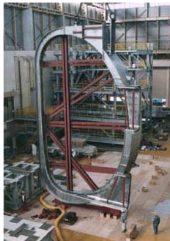
Figure 6. Many components and techniques that are needed for ITER have already been tested by industry, such as this full-scale vacuum vessel sector, produced in Japan (courtesy JEARI).
