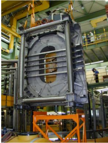
Figure 8. Many components and techniques that are needed for ITER have already been tested by industry, such as this model of the ITER Toroidal Coil, assembled in the Toska facility in Karlsruhe, Germany.
